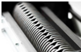
Specially hardened cutting rollers for precision cutting.
