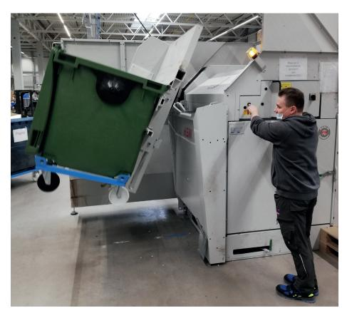
now conveyed in a tugger train, they are efficiently integrated into Alber's Intralogistics: a tugger train can pull four waste bins to the baling press at the same time. The result is a process which is four times as fast whilst also saving unnecessary trips. According to Alber, the whole concept works only because the HSM press fullfills the requirements so well.
