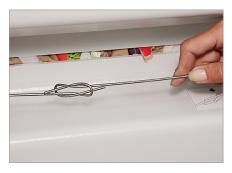
**Strapping** Manual bale strapping with Quick-link wire.
