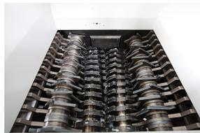
Stage 1: pre-shredding using a four-shaft system consisting of two intake shafts and two cutting shafts.
