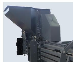
With large loading aperture for optimised feeding methods (1140 mm length)
