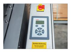
Functional operator control panel with LED indicator
