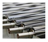
The induction-hardened, solid steel cutting rollers guarantee durability.
