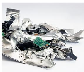
A conventional 3.5 inch hard disk is cut into at least three parts ("H-3 security cut"). The security level is thus many times higher than with conventional methods.
