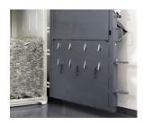
Special retaining claws optimize the compression of the pressing material.
