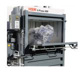
To fill the press, the upper half of the doors is folded down
