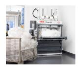
To fill the press, the upper half of the doors is folded down
