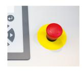
It may be necessary to stop the machine immediately so we have equipped the device with an emergency off switch which, when activated, will do just this.
