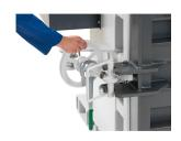
Hand wheel door lock - Easy to handle thanks to counter-rotating thread for quick opening and closing
