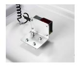
HSM TCS (Torsion Control System) for monitoring press ram movement
